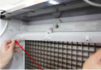
Hold left & right tabs in & pull distributor forward
