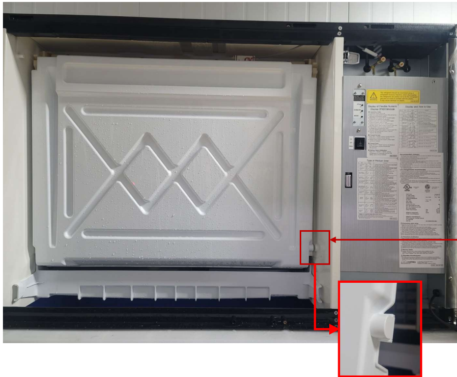
BIN SWITCH: MAGNET ON WATER CURTAIN. SWITCH IN CONTROL BOX.
