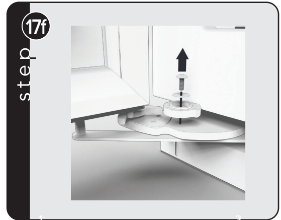
Remove the door cam screw, washer and door cam. Note the positioning of the cam to re-install after adjustment is completed
