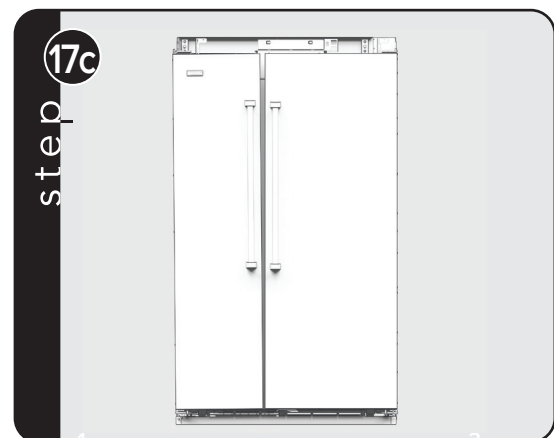
For uneven gap between two doors as shown in image follow step 17d
