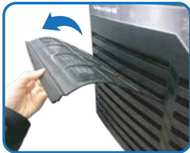
Remove air filter by sliding forward
