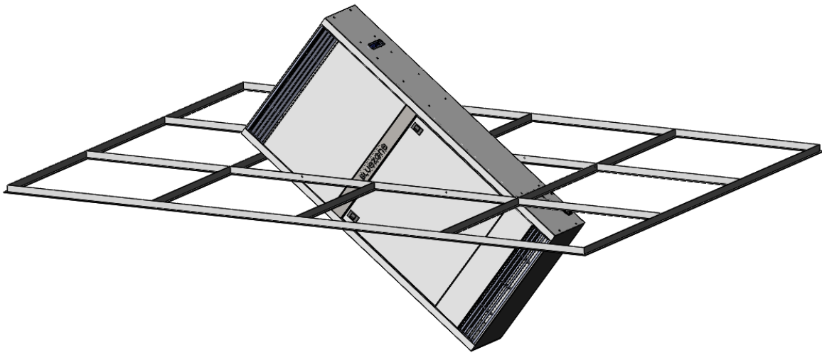
Figure 11: Insert the PK-220 Sideways and Upwards into the Ceiling Grid
