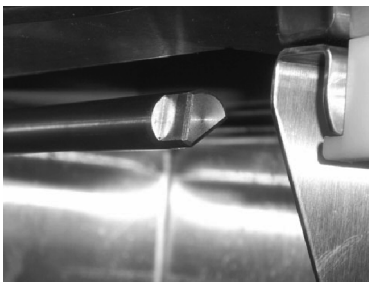
Figure-10: Door Alignment Arrow
