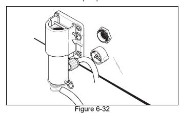
**Note:** Alignment of the air/mix pump is extremely important. Severe and costly damage may occur if it is not properly aligned.
