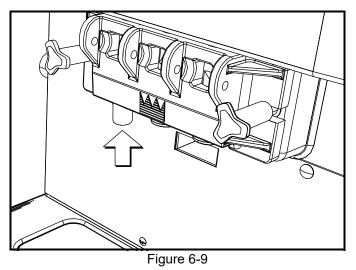
12. Slide the O-ring onto each pivot pin and lubricate.
