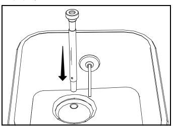
Figure 5-4 Feed Tube Position during Normal Operation
